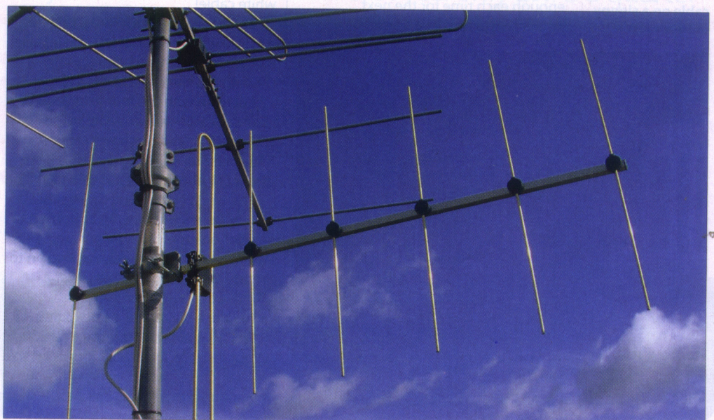
(below) Pole clash A Yagi aerial needs free space to work correctly
