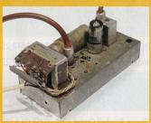
This 1950s distribution amplifier used an ECC84 low noise RF amplifier valve. The valves didn't last too long, and for a company with a lot of these amps in use the replacement schedule was like painting the Forth Bridge
