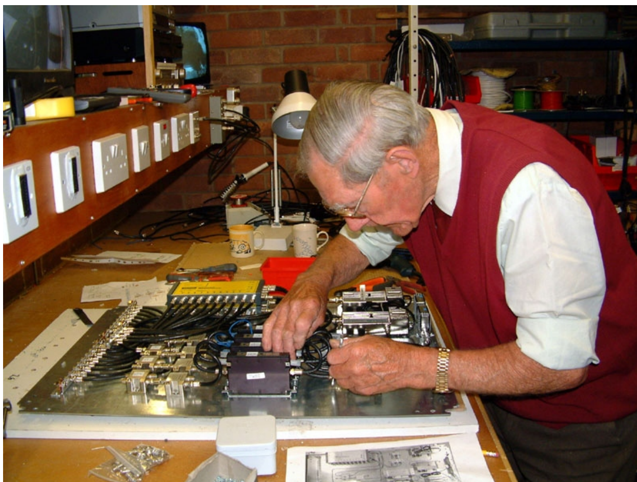
Fig 18. It's far better to plan, build, and test the head-end in advance. This engineer is 86 years old!
